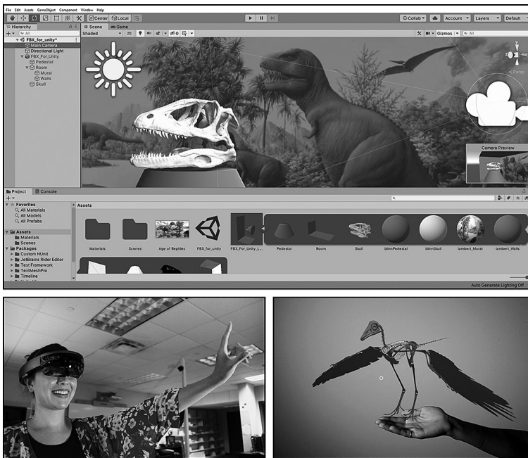
Figure 14.1 Top. Screenshot of a student's VR museum scene in the Unity game engine interface. Bottom left. Photo of a student using the HoloLens AR headset. Bottom right. Mixed reality photo of our Archaeopteryx 3D model, as captured by the HoloLens.
